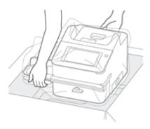
2. **Important**: Be sure to grab hold of the entire feeder, not just the moistener flap when lifting the device out of the box.
