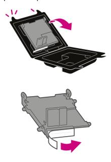
10. Squeeze the tabs and slide the printhead pegs into the lower set of grooves.
