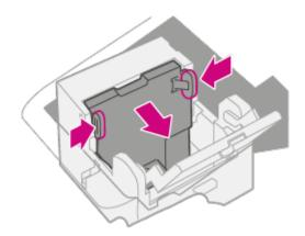
8. While squeezing, lift and tilt the printhead to the right. The printhead should come up out of the device.
