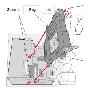
11. Keep squeezing the tabs and push the printhead flush against the wall. Tabs will snap outward when placed correctly.
