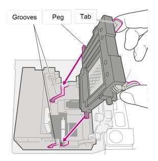
6. Keep squeezing the tabs and push the printhead flush against the wall. The tabs snap outward when you place the printhead correctly.
