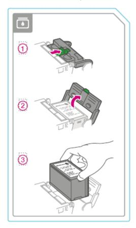
6. Insert the new ink cartridge, then close the ink cartridge guard.
