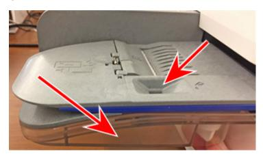
2. Slide the envelope flap under the edge of the feed deck when inserting an envelope. Otherwise, the moistener cannot wet the flap.
