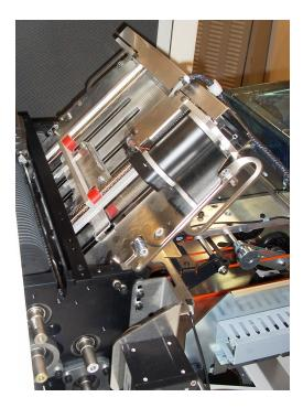
**Auto Buckle Chute Reinstalled**
