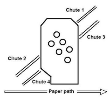
You can only access the auto buckle chutes by opening the folder and side access covers. These covers are interlocked, so the machine stops when the covers are open and will not restart until you close them.
