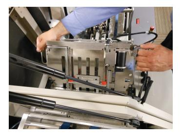
4. Move the chute from side to side to be sure it's securely in place. If the hole on the side of the latch handle is showing, the chute is not fully engaged (like in first image here). When the chute is installed right, it should look like the second image.
