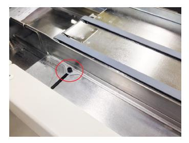
Prefeed Deck Side Guide Locking Screws (three in total, one visible in this photo)
