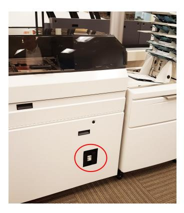
Power Switch on the Pulse Input
