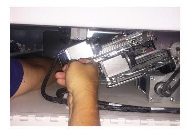
5. Move the chute from side to side to be sure it's securely in place. If the hole on the side of the latch handle is showing, the chute is not fully engaged (like in first image here). When the chute is installed right, it should look like the second image. (These images show upper chutes, but it's the same concept for lower chutes.)
