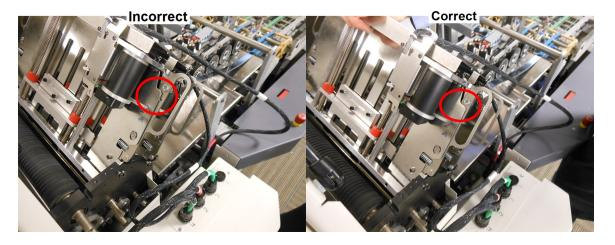
Latch NOT Engaged (incorrect) and Latch FULLY Engaged (correct)
