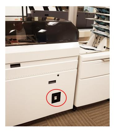
Power Switch on the Pulse Input
