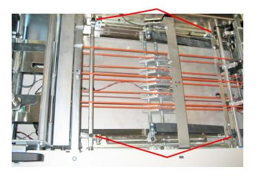
**Lock Screws on Accumulator Sides**
